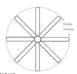
**DIMENSIONS** Blade Sweep: 56" H: 15" (Using 6" Rod)
